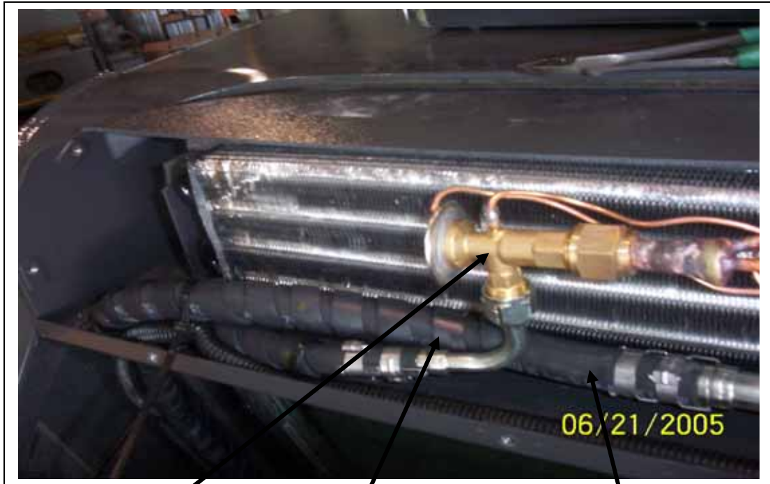
5/16" hose to receiver drier.
