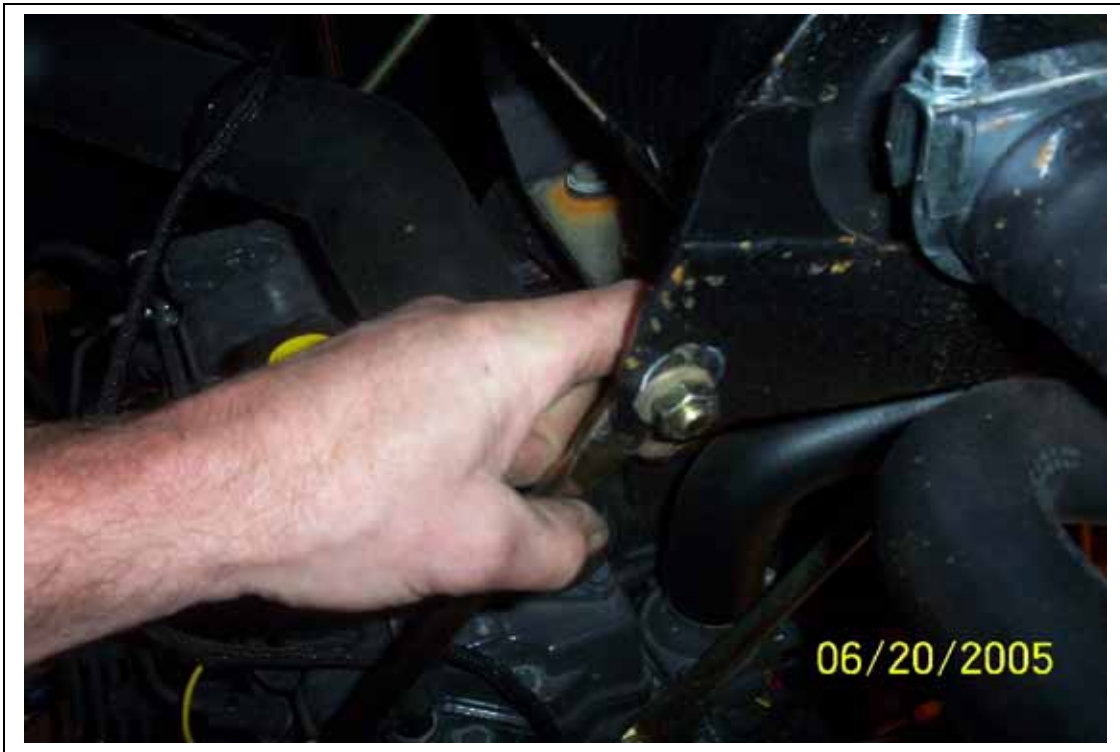
Loosen bracket from front of engine to muffler support. Temporarily remove.
