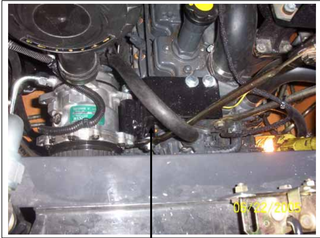
Exhaust bracket re-installed. Washers may be required to obtain proper alignment.
