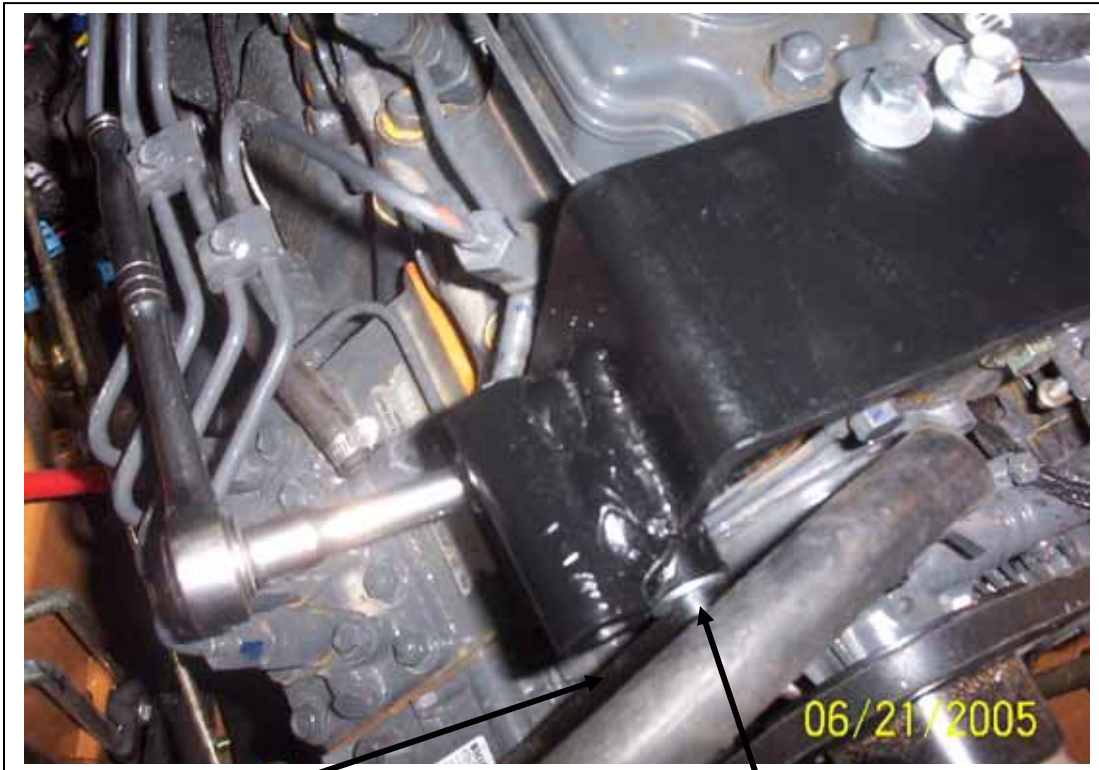
Tightener bracket for compressor.
